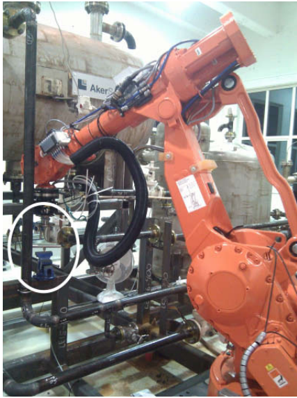
Fig. 6. The max torque test setup comprise an industrial robot that turns the same type of needle valves used during the on-site demonstrations.
