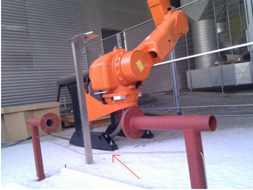
Fig. 10. The result of the crash test where the robot is run into a 6 mm thin pipe (red arrow) with a speed of 30 cm/s.
